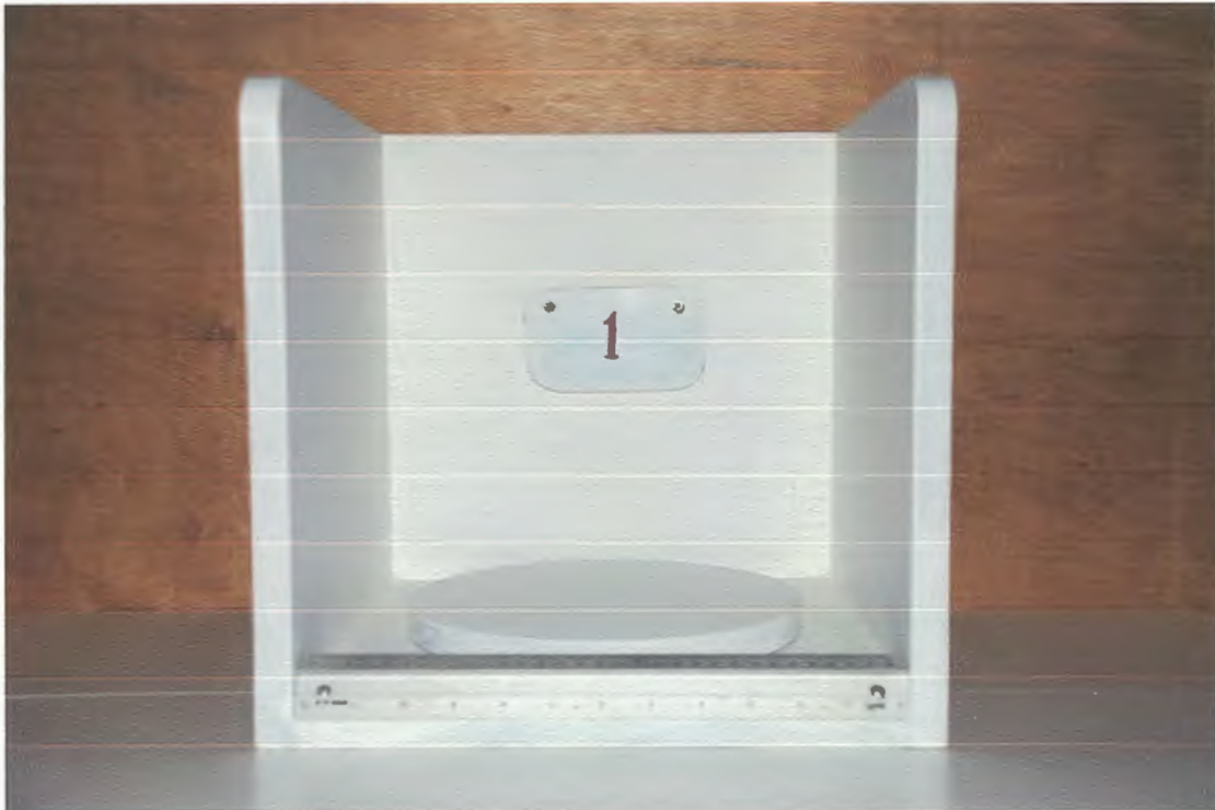
Plate 15:- The Calibrated photographic box, build specifically for this study.
