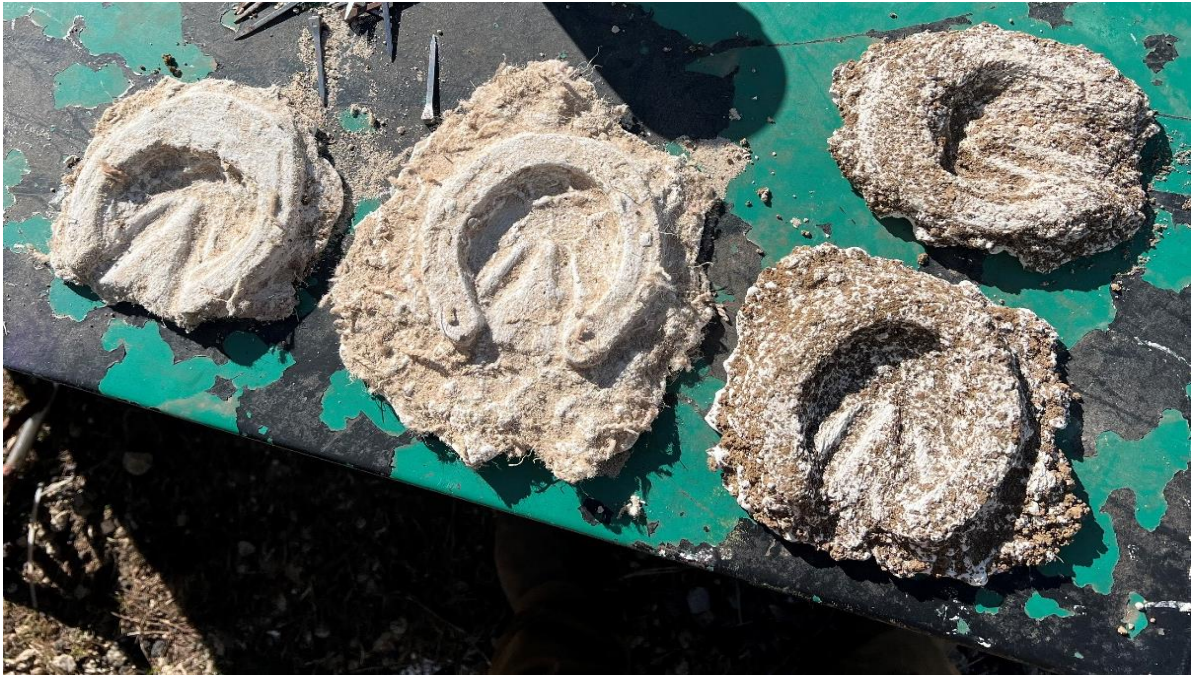
FIGURE 12: An example of the casting method used to demonstrate shoe penetration depth (see Appendix A.1).
