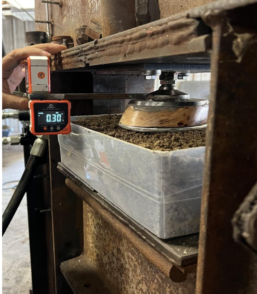
FIGURE 11: The wooden foot in a hydraulic press (see Appendix A.1).
