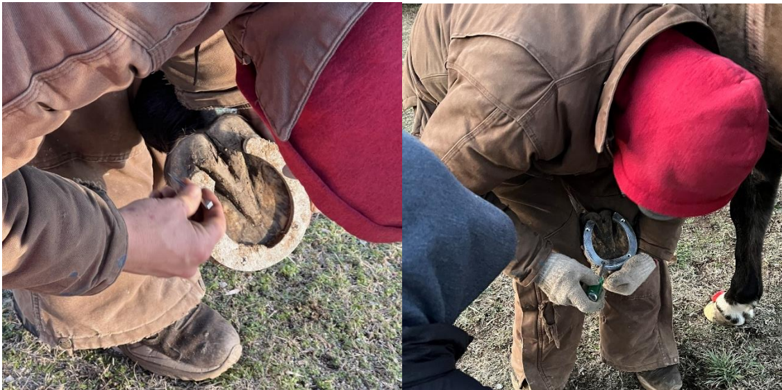
FIGURE 17: (Left) This photo is post-measurement; the Pam prevents dirt from sticking in the shoe. (Right) A new test shoe being applied to the base shoe (see Appendix A.1).
