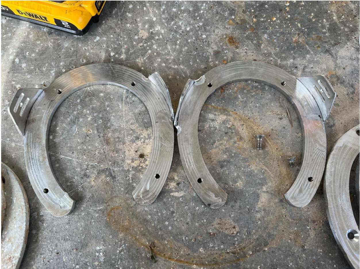
FIGURE 5: The Base Shoe with Hanton System™ clips welded on and ready for application (see Appendix A.1).
