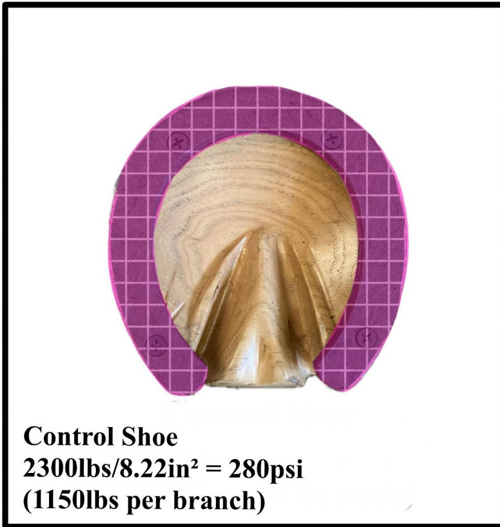
FIGURE 1: A control shoe showing perfectly even load distribution (see Appendix A.1).
