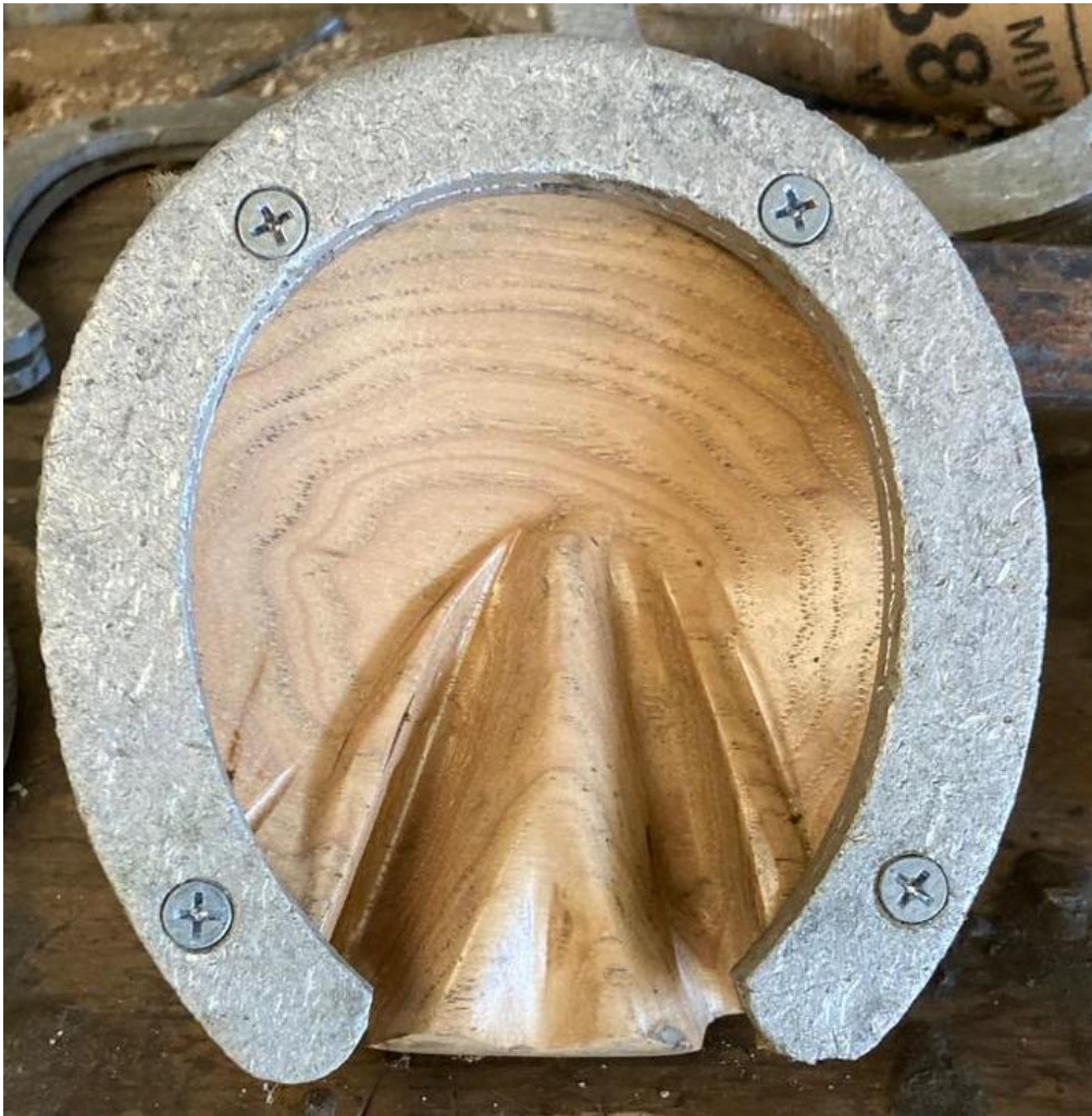
FIGURE 10: The wooden foot with the Base Shoe applied (see Appendix A.1).
