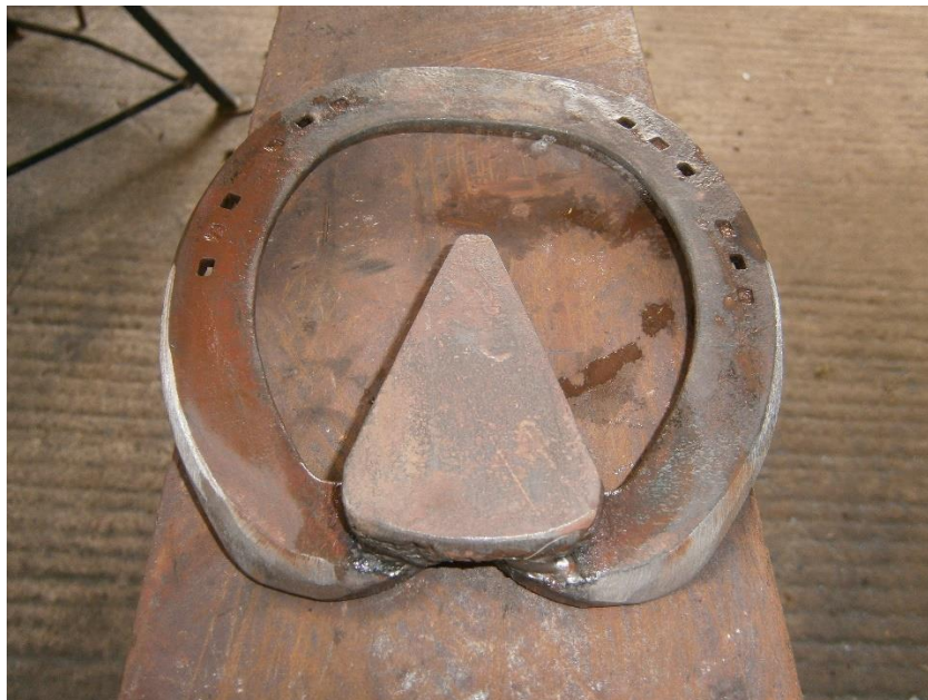
Figure 12: A removed shoe demonstrating the height of the insert required to obtain sufficient frog contact.
