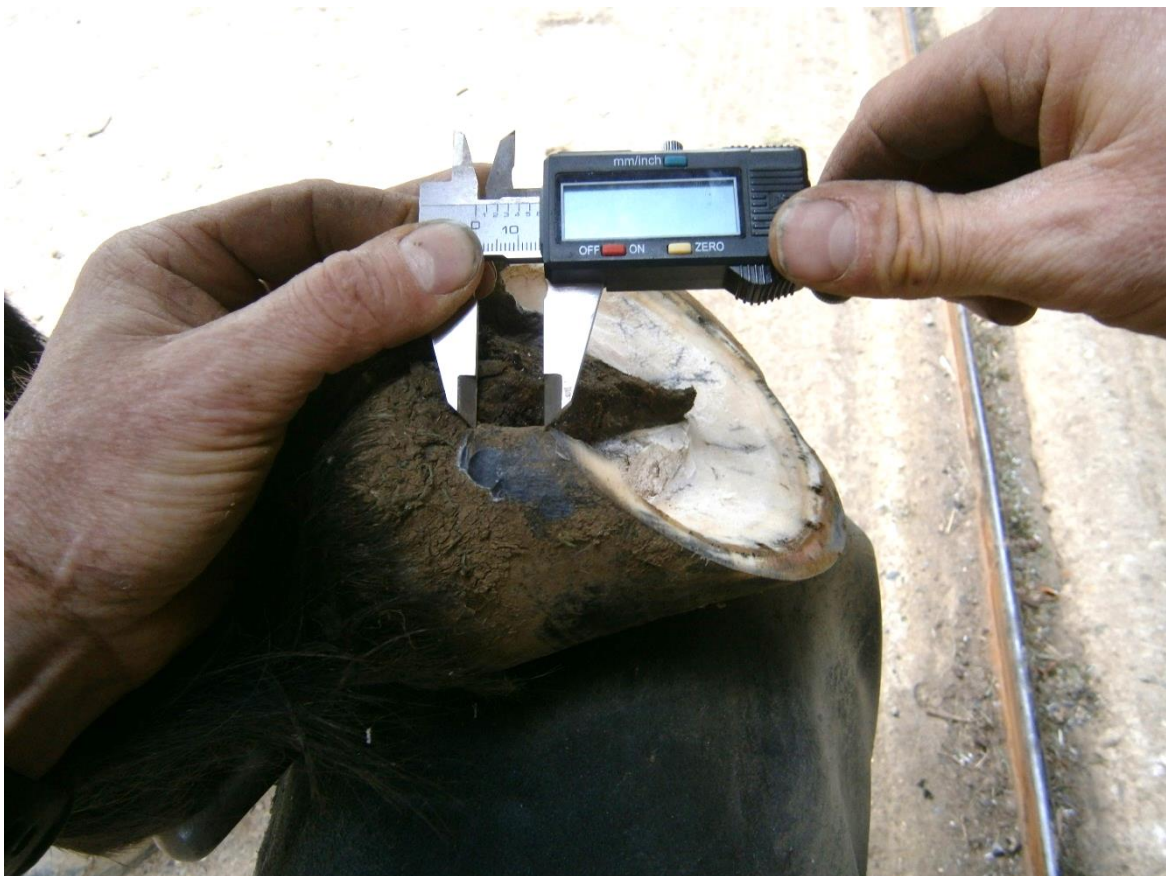
Figure 7: Heel height measurements were taken manually using the professional Vernier digital calipers.
