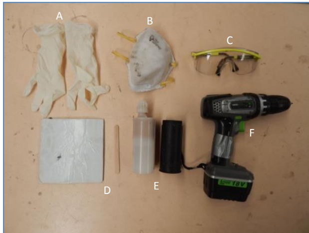
Figure 1: Marking equipment and PPE. A. Gloves B. Dust mask C. Eye protection D. Mixing pallet and spatula E. Acrylic hoof rebuild compound (glue) F. Battery operated hand held drill and bit
