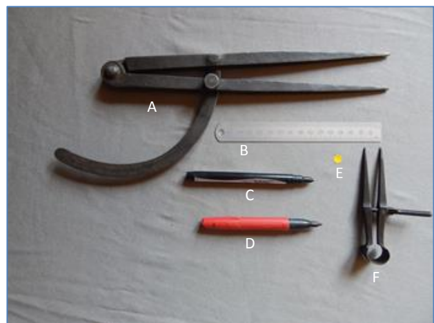
Figure 2: Measuring and recording equipment. A. Large Compass B. Engineers ruler C. Fine line marker pen D. Regular marker pen E. 8 mm Sticker disc F. Small compass
