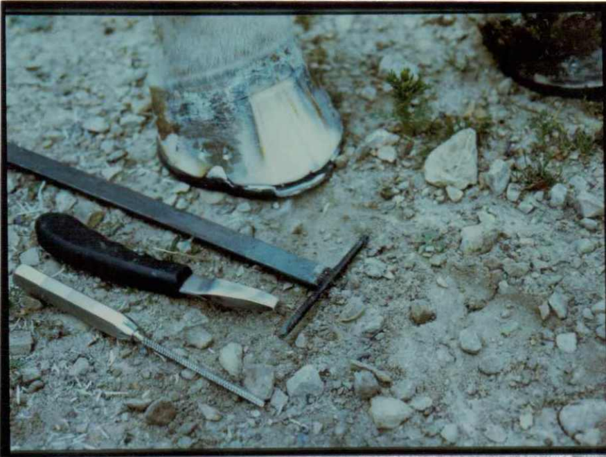
Fig. 14. Shows shoe fitted in place and tool designed for grooving i.e. a 4" nail welded to a flat bar, heated and burnt in the hoof. Afterwards well cleaned with veterinary grooving knife.
