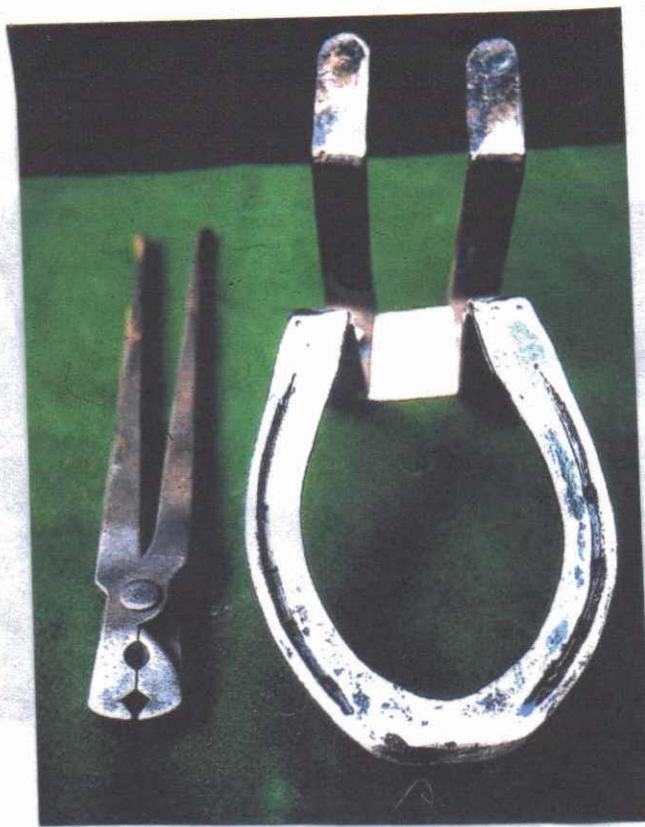
Nail Pullers for the removal of individual Nails from the fullering avoiding any stress on the leg.
