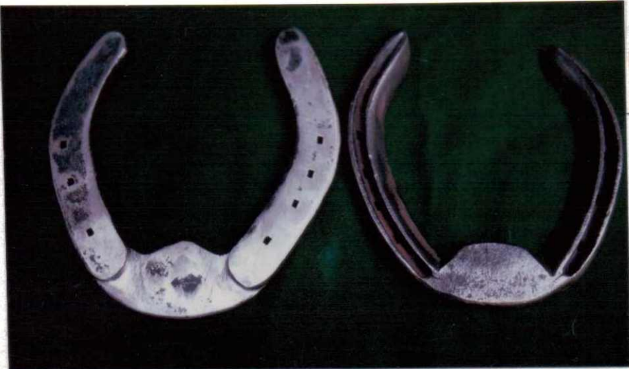
Shows type of shoe suitable for use in the case of Horn Tumour. Fig. 9.
