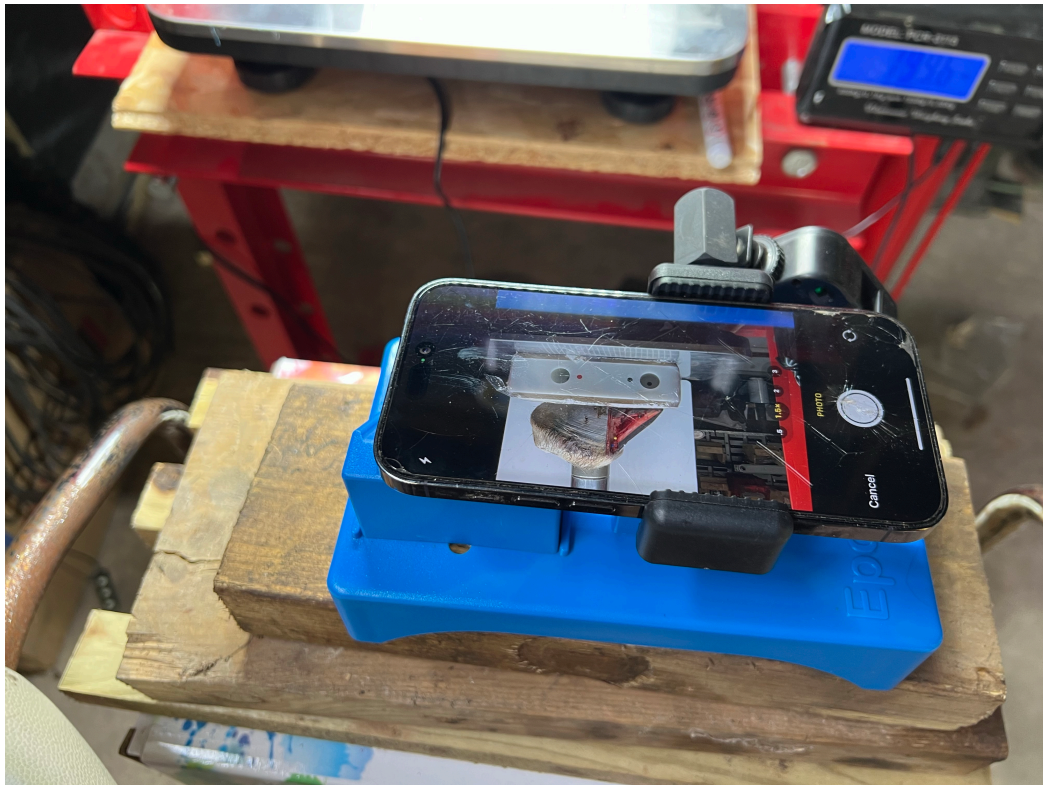
Figure 12: The Epona 6 camera holder holding an iPhone 14 pro 2 , showing the image just taken.
