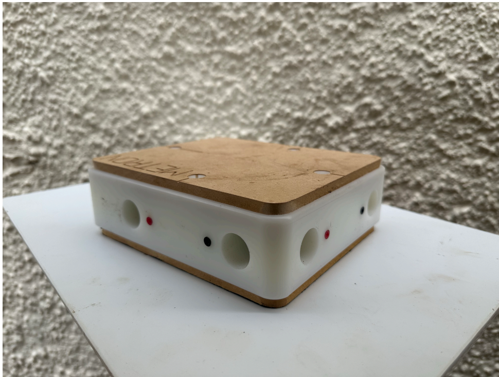
Figure 13: The Metron 6 blocks various different screws and holes. The software uses their distances and depths to calibrate the image.
