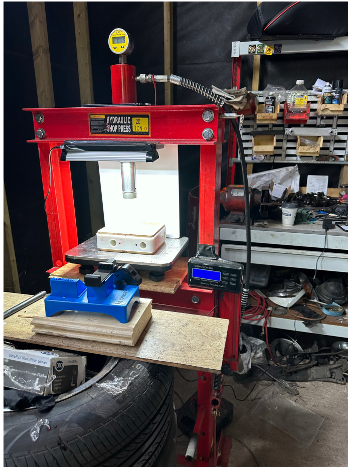
Figure 9: The set up for conducting the study consisting of; the press, Metron 6 block, ONPNO weighing scales 1 , LED 3 lighting bar and the Epona 6 camera holder.
